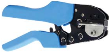
KC8C48 For Non-Insulated Receptacle & Tab Terminal AWG 20-18/18-14/12-10 0.5-1/1-2.5/4-6 mm 2
