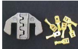
C DIE Open Barrel Terminal AWG 20-18/16-14/12-10 0.5-1.0/1.5-2.5/4.0-6.0 mm 2
