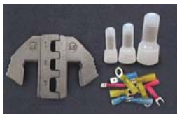
A5 DIE Closed End Connector & Heat Shrink Terminal AWG 22-16/16-14/12-10 0.5-1.5/1.5-2.5/4.0-6.0 mm 2
