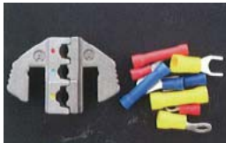
A DIE Insulated Terminal AWG 22-18/16-14/12-10 0.5-1.0/1.5-2.5/4.0-6.0 mm 2
