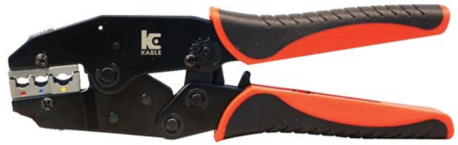
KC-6IA For Insulated Terminal AWG 22-18/16-14/12-10 0.5-1/1.5-2.5/4-6 mm 2
