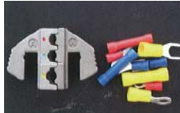
A DIE Insulated Terminal AWG 22-18/16-14/12-10 0.5-1.0/1.5-2.5/4.0-6.0 mm 2
