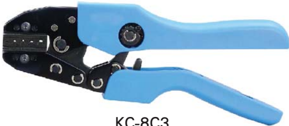
KC-8C3 For Non-Insulated Receptacle & Tab Terminal AWG 26-22/20-18/16 0.14-0.25/0.5-1/1.5 mm 2
