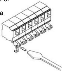
2. Insert the wire (up to 2.5 mm<sup>2</sup> /single core) in the corresponding connection hole while keeping the pressure on the lever.
